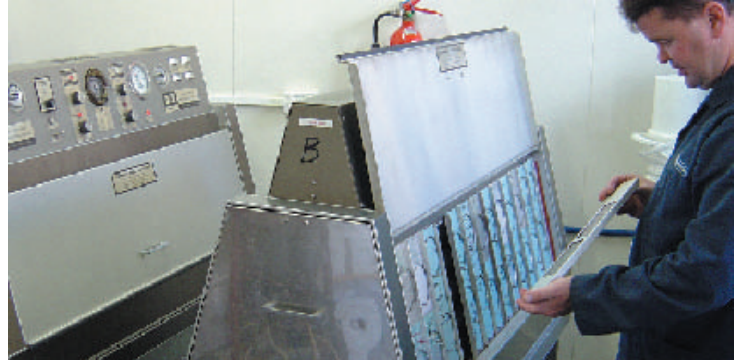
AHI Roofing's Accelerated UV Exposure testing station.
